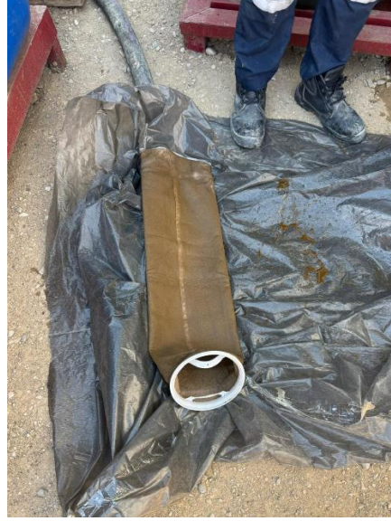
Figure 1 — Dirty filter bag after filtered-circuit recirculation. Particle load exceeded filter capacity.
